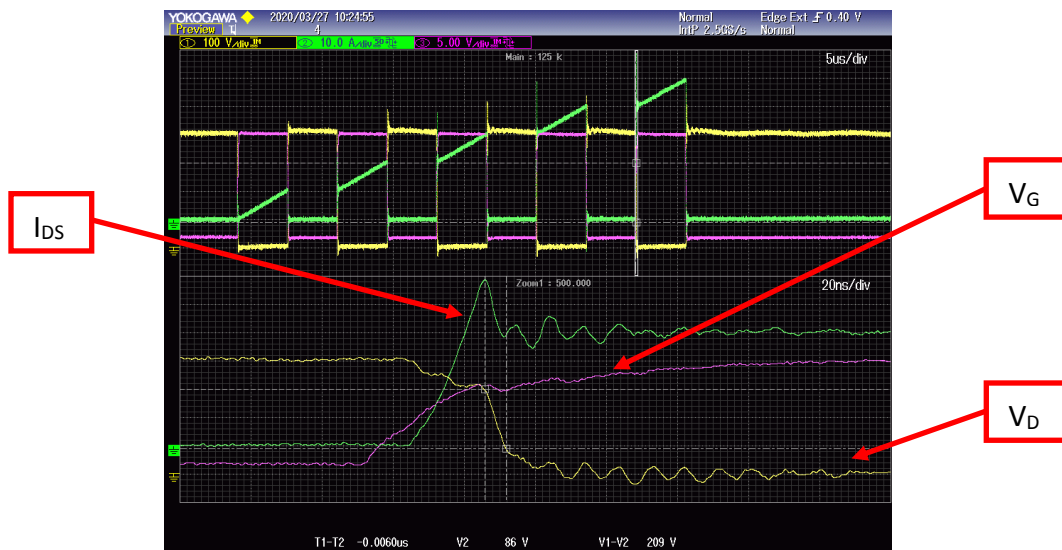
Figure 25. Double pulse waveforms
