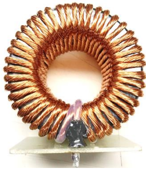
Figure 22. Synchronous Boost Inductor
