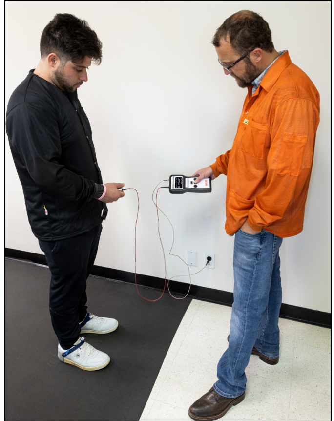
Figure 10. Using the SCS 770765 Handheld Electrode to measure Floor Materials and Footwear - Resistance Measurement in Combination with a Person (ANSI/ESD STM97.1)
