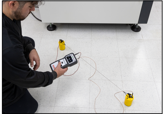
Figure 13. Measuring the Resistance Point-to-Point (R tt ) of floor materials
