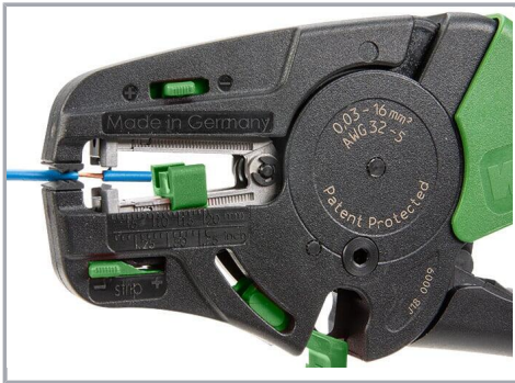
Partially stripping a conductor.
