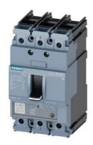
circuit breaker 3VA5 UL frame 125 breaking capacity class M 35kA @ 480 V 3-pole, line protection TM230, FTAM, In=80A overload protection Ir=80A fixed short-circuit protection Ii=5...10 x In UL489 SB (naval), 50 deg. cel. cable connection on both sides
