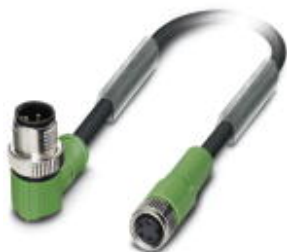
Sensor/actuator cable, 4-position, Variable cable type, Plug angled M12 SPEEDCON, A-coded, on Socket straight M8, cable length: Free input (0.2 ... 40.0 m)
