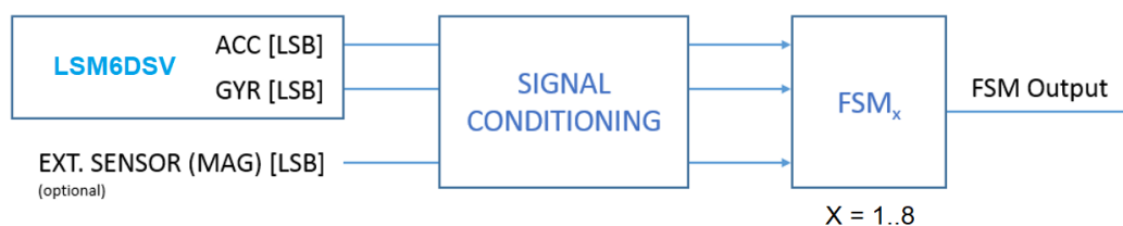
Figure 3. State machine in the LSM6DSV
