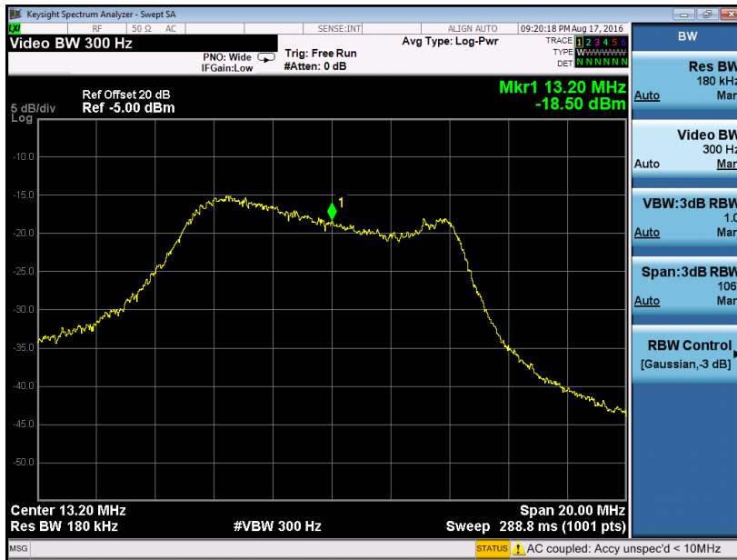
Figure 3. IF filter Center Frequency = 13.2MHz when FCEN is 001101, FBW is 01, and FCENMSB is 0 in Test Mode 2 register.
