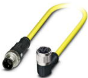
Sensor/actuator cable, 3-position, PVC, yellow, Plug straight M12 SPEEDCON, A-coded, on Socket angled M12 SPEEDCON, A-coded, cable length: 0.5 m
