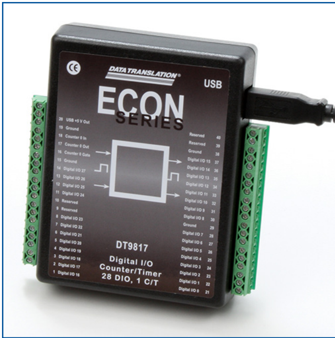
Connect to a host computer using the standard USB 1.1 or 2.0 plug-in connector on the ECONseries module. The USB connector provides power to the module, eliminating the need for an external power supply, while providing complete enumeration for all data flow.
