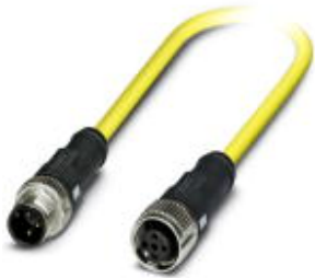
Sensor/actuator cable, 3-position, PVC, yellow, Plug straight M12 SPEEDCON, A-coded, on Socket straight M12 SPEEDCON, A-coded, cable length: 1.5 m
