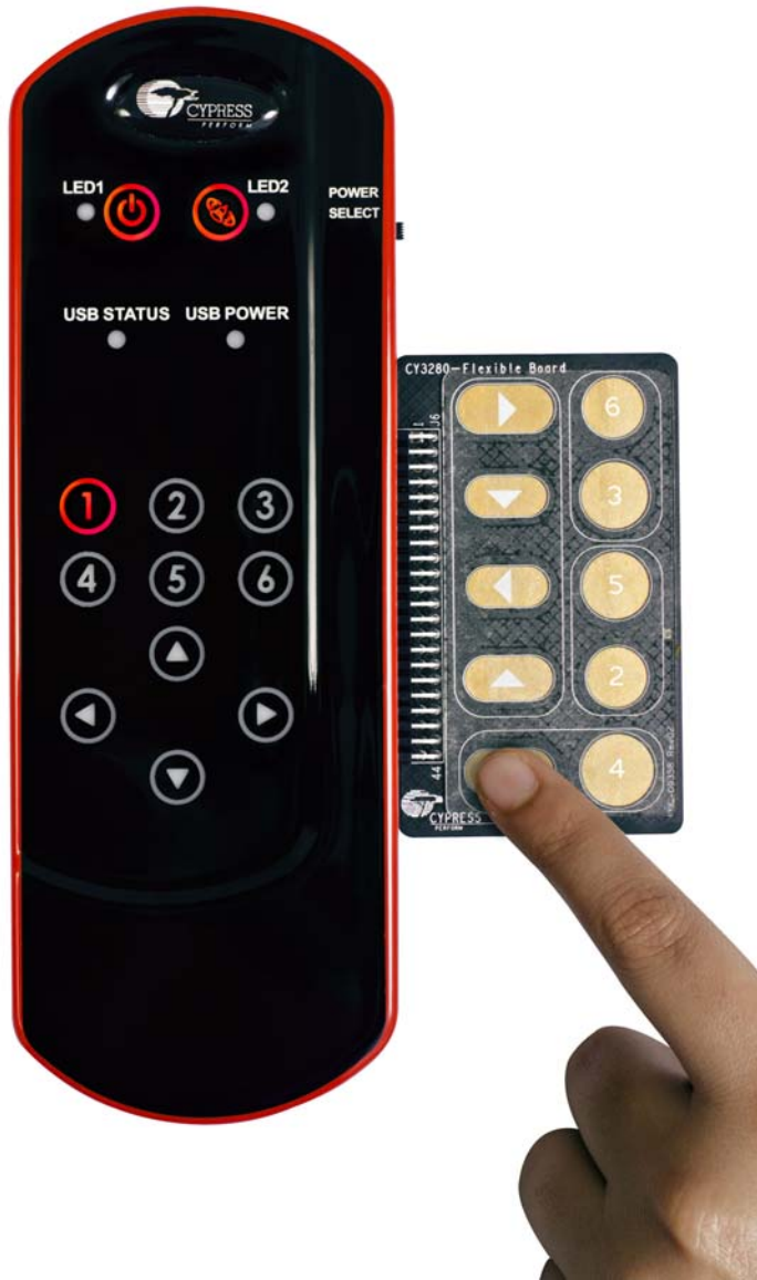
Figure 3-3. Demonstration of SmartSense Auto-Tuning with Flex-PCB
