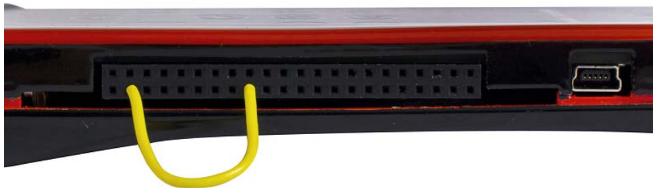
Figure 3-25. Shorting Button #6 (pin #27) to Vdd (pin #41)
