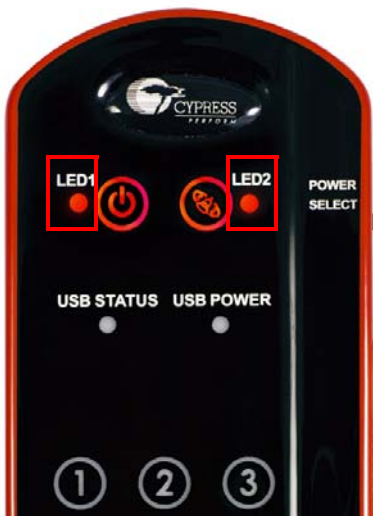
Figure 3-16. Host Controlled GPO LEDs
