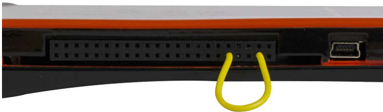
Figure 3-23. Shorting Button #5 (pin #3) to Button #2 (pin #9)
