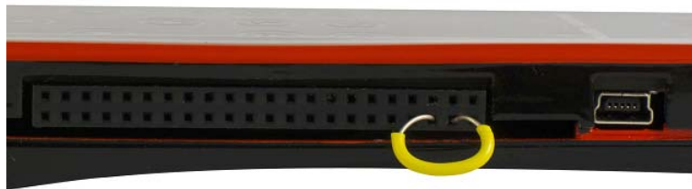
Figure 3-21. Shorting Button #5 (pin #3) to Ground (pin #5)
