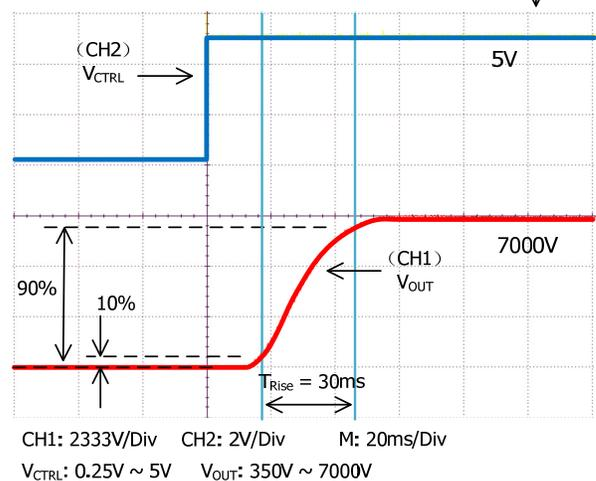
Figure 12. Rising Trail for Large Signal Response
