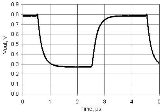
Figure 11-52. VDAC Step Response, Codes 0x40 - 0xC0, 1 V Mode, Fast Mode, V DDA = 5 V
