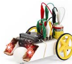
ADD SOME HEADLIGHTS USING ZIP HEX LEDs
