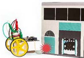
USING THE ACCELEROMETER TO DETECT AN IMPACT
