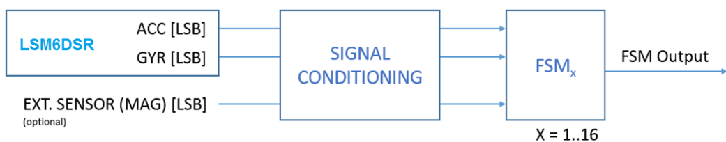
Figure 2. State machine in the LSM6DSR
