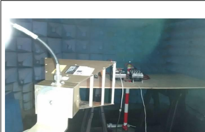
Figure 3: Radiated Immunity Test Set up
