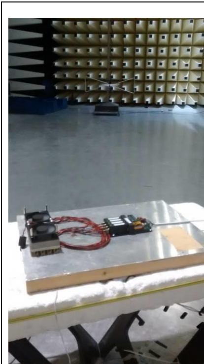
Figure 1: Radiated Emissions Test Set up
