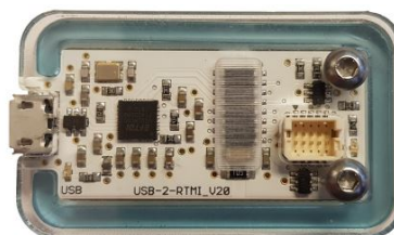
Figure 3: USB-2-RTMI v20 with galvanic isolation
