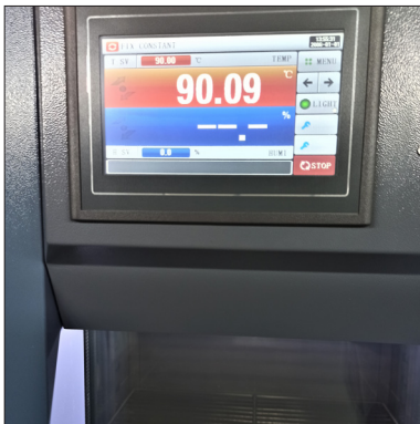
Temperature set in the climatic chamber
