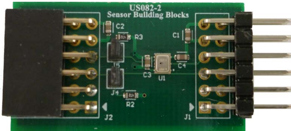
Figure 1. US082-HS3001EVZ Pmod Board
