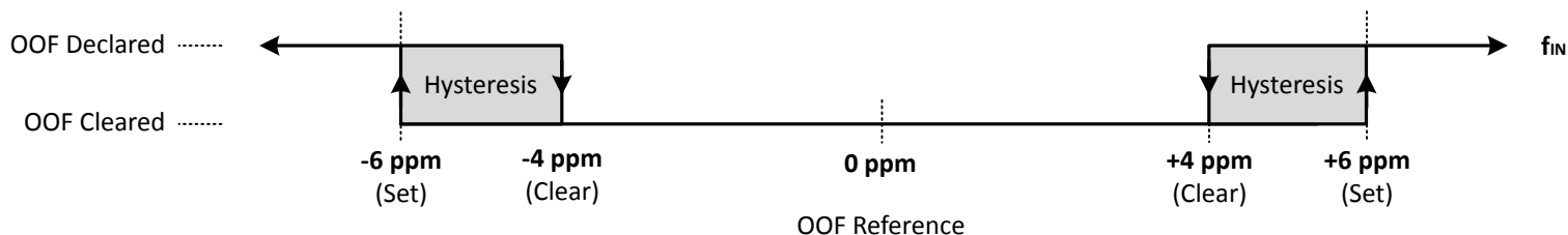
Figure 4.13. Example of Precise OOF Monitor Assertion and De-assertion Triggers
