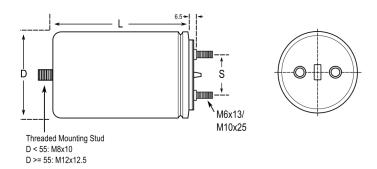
General Information Series C44A Dielectric Metallized Polypropylene Style RoHS With Exemptions **REACH** SVHC (Pb - CAS 7439-92-1) SCIP Number cc1c1ec4-db9e-4815-b26b-e8a34ddfb776 Lead Threaded Studs M6 AEC-Q200 No Component Weight 375 g Thermal Resistance = 2.6 C/W. Miscellaneous
