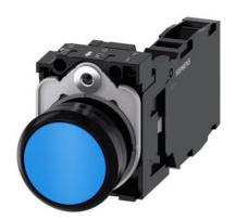
Pushbutton, 22 mm, round, plastic, blue, pushbutton, flat, momentary contact type, with holder 1 NO+1 NC, screw terminal, with laser labeling, upper case
