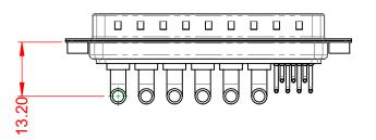
POWER/CO-AX CONTACT RATING:40A (CURRENT)(IF PRESENT)SIGNAL CONTACT CURRENT RATING:5A PER CONTACTSIGNAL CONTACT RESISTANCE: $10m\Omega$  MAX.INSULATOR RESISTANCE:5000MΩ min.DIELECTRICDIELECTRIC
