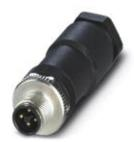
Power connectors, Power, 4-position, Plug straight M12, T-coded, Screw connection, knurl material: Zinc diecast, nickel-plated, cable gland Pg11, external cable diameter 8 mm ... 10 mm, For direct current up to 12 A/63 V, Contact 4 leading
