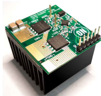
Figure 13. NCP51820 HB GaN Driver EVB and Heatsink
