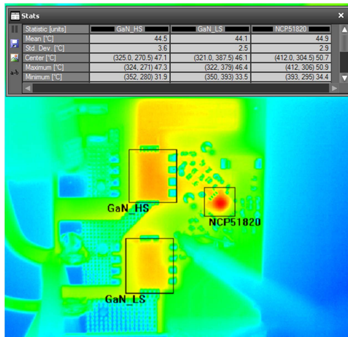
Figure 19. Thermal Image: FAN7688 LLC/NCP51820 HB GaN Driver EVB, 400 VIN, 100 kHz, 12.5 V, 20 A
