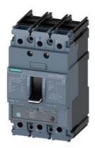
circuit breaker 3VA5 UL frame 125 breaking capacity class S 25kA @ 480 V 3-pole, line protection TM240, ATAM, In=50A overload protection Ir=40A ...50A short-circuit protection Ii=5...10 x In nut keeper kit on both sides
