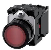
Illuminated pushbutton, 22 mm, round, plastic, red, pushbutton, flat, momentary contact type, with holder, 1NC, LED module with integrated LED 110 V AC, screw terminal, with laser labeling, upper case and lower case, always upper case at beginning of line
