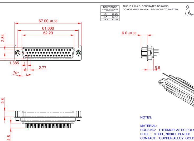
HOUSING: THERMOPLASTIC POLYESTER, UL94V-0 CONTACT: COPPER ALLOY, GOLD FLASH PLATED OPERATING TEMPERATURE: -55°C to +105°C
