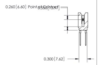
745 Series Ultra-Mate Card Edge Connector - Press Fit Part Number: 745-102-540-206
