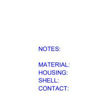
THERMOPLASTIC POLYESTER, UL94V-0 STEEL, NICKEL PLATED COPPER ALLOY, 30µ" GOLD PLATED
