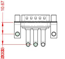
40A (CURRENT) POWER/CO-AX CONTACT RATING: (IF PRESENT) SIGNAL CONTACT CURRENT RATING: 5A PER CONTACT SIGNAL CONTACT RESISTANCE:  $10m\Omega$  MAX.
