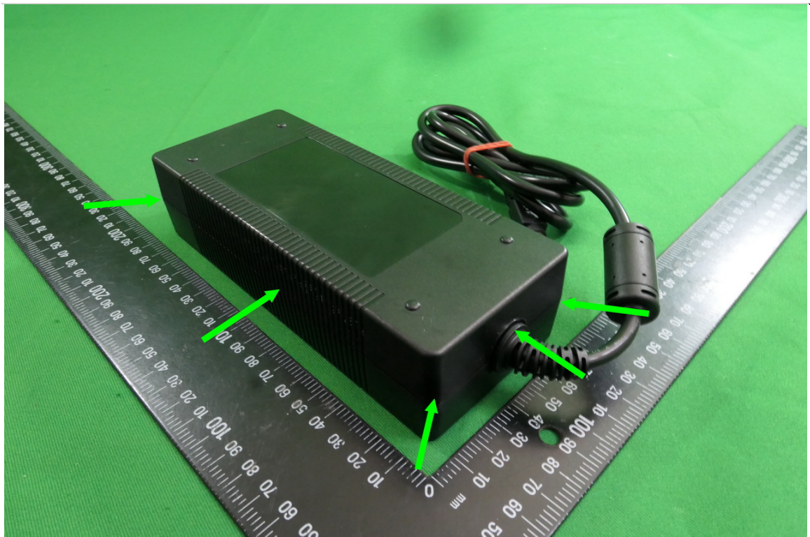
View of Discharge Point -2 (Green: Air Discharge)
