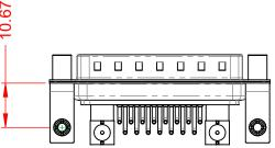
75Ω (IMPEDANCE) POWER/CO-AX CONTACT RATING: (IF PRESENT) SIGNAL CONTACT CURRENT RATING: 5A PER CONTACT SIGNAL CONTACT RESISTANCE:  $10m\Omega$  MAX. **INSULATOR RESISTANCE:** 5000MΩ min.
