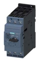
Circuit breaker size S2 for motor protection, CLASS 10 A-release 49...59 A N-release 845 A screw terminal increased switching capacity
