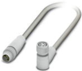
Sensor/actuator cable, 4-position, PP-EPDM halogen-free, gray RAL 7035, Plug straight M8, on Socket angled M8, cable length: 1.5 m, Hygienic design, with plastic knurl
