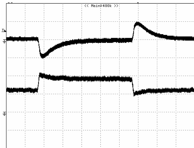
Figure 8: Output voltage response to step-change in load current (75%-50%-75% of I_o , max; di/dt = 0.1A/\mu s ). Load cap: 10\mu F tantalum capacitor and 1\mu F ceramic capacitor. Top Trace: V_{out} (0.2V/div, 200us/div), Bottom Trace: I_{out} (1A/div). Scope measurement should be made using a BNC cable (length shorter than 20 inches). Position the load between 51 mm to 76 mm (2 inches to 3 inches) from the module
