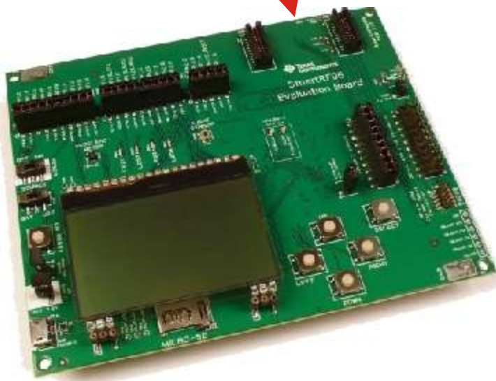
SMART RF06 Evaluation board (TI)
