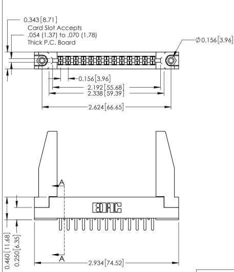
0.295 [7.49] Card Slot  $\forall$ - $\forall$ SECTION 0.165[4.19] Point of Contact
