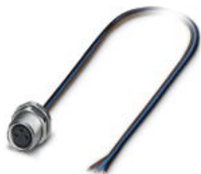
Sensor/actuator flush-type socket, 3-pos., M8, rear/screw mounting with M10 thread, with 0.5 m TPE litz wire, 3 x 0.25 mm 2
