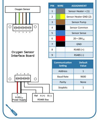
**4b. Analogue variants:** Connect power and input/output connections to the interface board.
