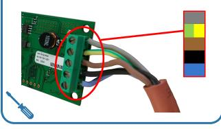
**4a. RS485 variant:** Connect power and input/output connections to the interface board.
