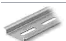
Item no.: 210-112 Steel carrier rail; 35 x 7.5 mm; 1 mm thick; 2 m long; slotted; according to EN 60715; "Hole width 25 mm; silver-colored
