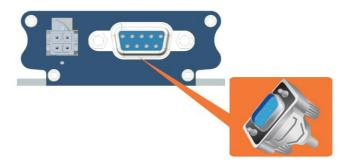
Connect the RS-232 DB-9 serial cable and secure the connection by tightening both thumb knobs on the connector.
