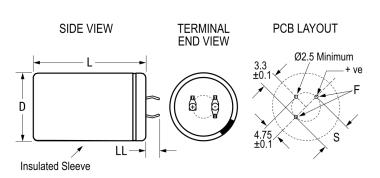
General Information Series ALC80 Dielectric Aluminum Electrolytic Description Snap-In, Aluminum Electrolytic RoHS Lead 3 Pin Short AEC-Q200 No Halogen Free Yes 60 g Component Weight Notes Dimensions D And L Include Sleeving. Shelf Life 156 Weeks
