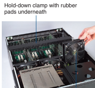
Three 114 CFM hot-swappable cooling fans
