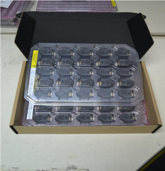
Figure: Shows the Tray packing into the box. Each box consist of 3 trays. Each tray consist of 10 units each. Quantity- Total 30 units per box.
