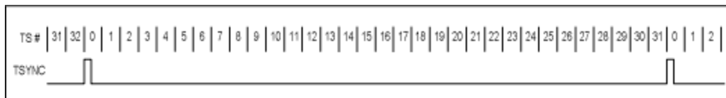
Figure 2. Transmit-side timing between TSYNC and time slot (TS) number.
