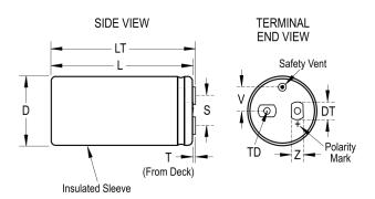
General Information Series ALS80 Dielectric Aluminum Electrolytic Description Screw Terminal, Aluminum Electrolytic RoHS AEC-Q200 No Halogen Free Yes Component 300 g Weight Dimensions D And L Include Sleeving. MS (MxH) = Notes M12x16. Mounting Clamp (Sold Separately): V4/2737 Shelf Life 156 Weeks
