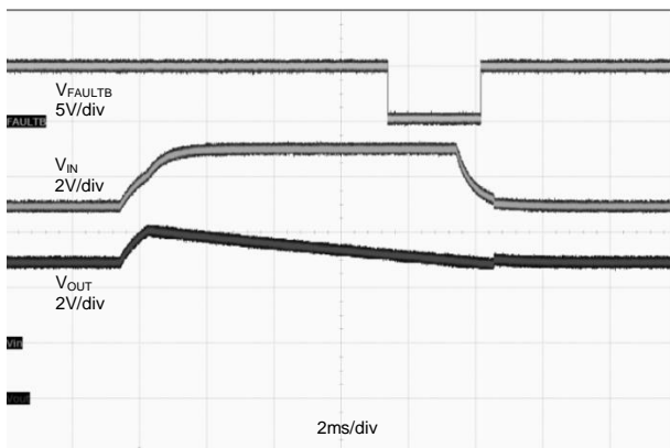
Figure 18. Input Overvoltage Protection and Recovery V_{IN} = 5 - 7 - 5\text{V} , R_{VLIM} = 56\text{k}\Omega , Load = 1\text{k}\Omega
