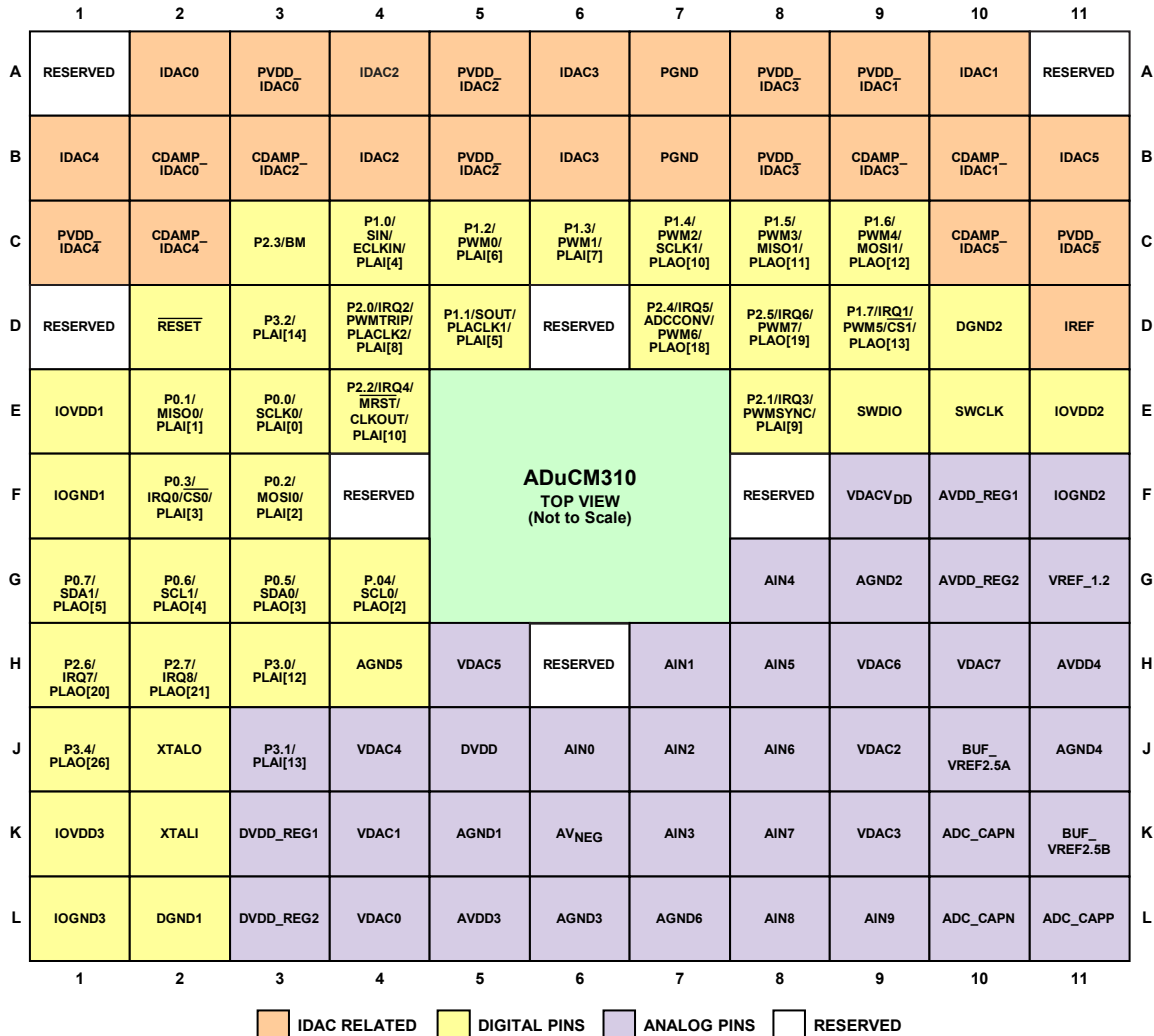
Figure 7. Pin Configuration
