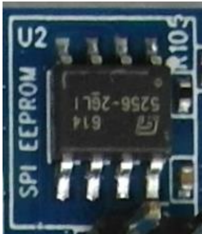
Figure 16: SPI EEPROM schematic and PCB
