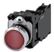
Illuminated pushbutton, 22 mm, round, Metal, shiny, red, pushbutton, flat, momentary contact type, with holder, 1 NO+1 NC, LED module with integrated LED 230 V AC, spring-type terminal, with laser labeling, upper case and lower case, always upper case at beginning of line
